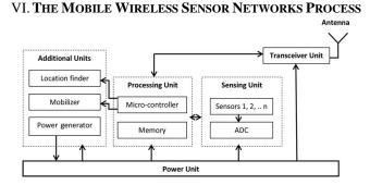
Sensor terminals include one or more sensors (i.e. temperature, light, humidity, humidity, pressure, luminosity, proximity, etc.), microcontroller, external memory, radio transceiver, analog to digital converter (ATC), antenna and battery. Again, board storage, battery power, processing, and radio capacity are limited due to the small size of the terminals [15].
