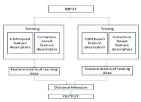
Figure 3.1.1: System Architecture For Image Retrieval
