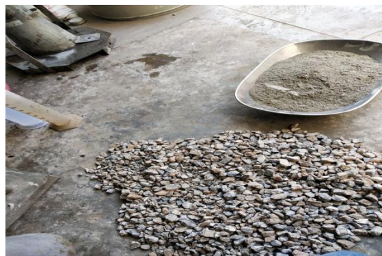
Fig. 2. Ingredients to make pervious concrete using RCAs
