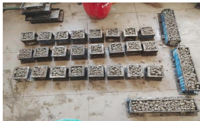
Fig. 3. Casting of specimens before placing it into curing tank
