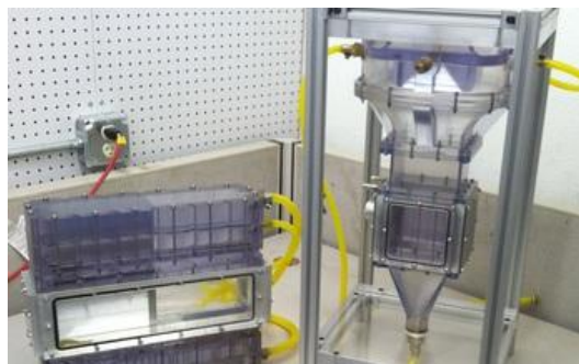
Fig. 4 Flo Design Sonics created AWS to clean water that rises to the top during gaseous petrol extraction by pressure-driven breaking (otherwise called fracking). The organization built up a test framework that can clean water streaming
