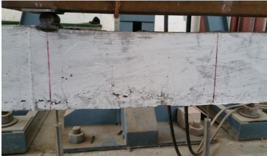
Figure 13 Failure Pattern in RC Beam
