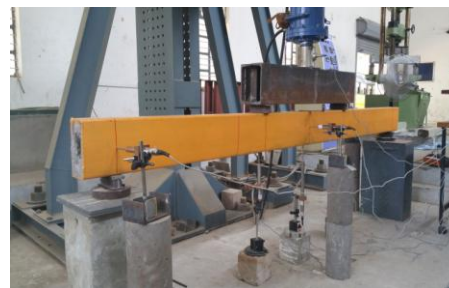
Figure 5. Testing of CFDST Beam
