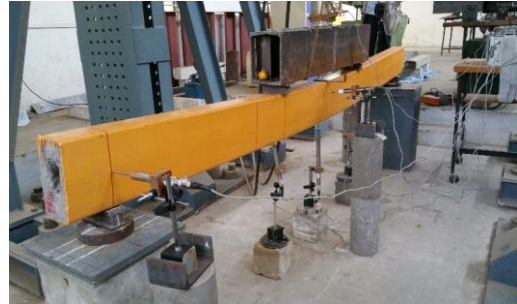
Figure 14 Failure Pattern in CFDST Beam
