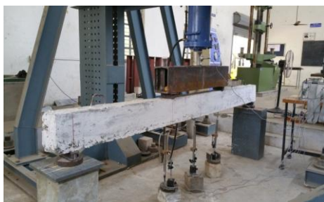
Figure 4. Testing of RC Beam
