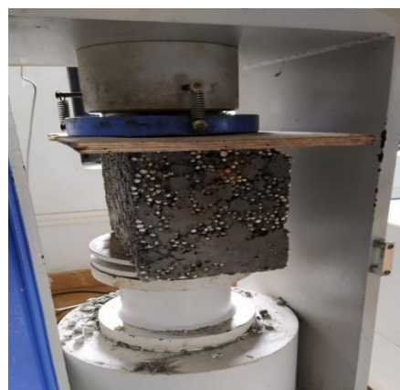
Fig 9 Compression Test on Polystyrene block
