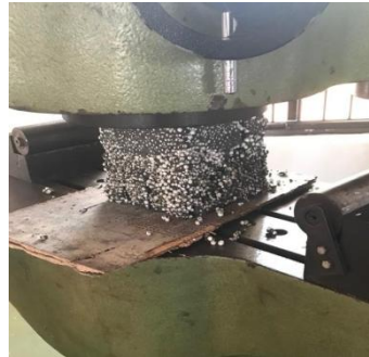
Fig 3. Compression test on polystyrene cubes
