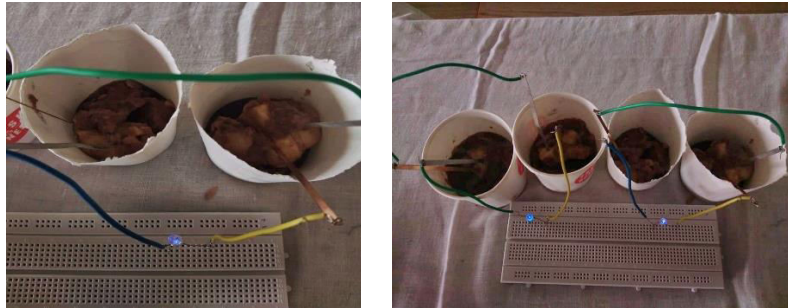
Fig 10: Lighting up of LEDs using two and four electrode pairs respectively
