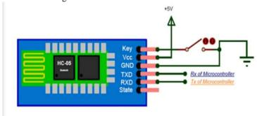
During power up the key pin can be grounded to enter into Command mode, if it is left free it by default it will enter into the data mode. Once the module is powered we should be able to discover the Bluetooth device as "HC-05" and then connect with it using the default password 1234 and start communicating with it. The default parameters such as name password and other parameters can be changed by entering into it.
