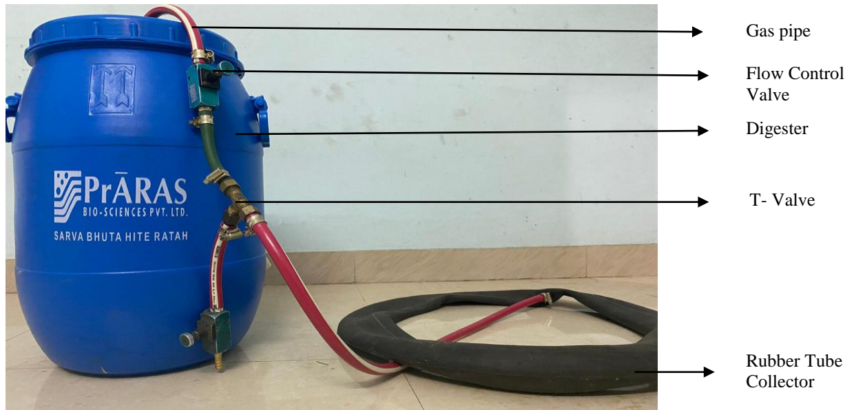
Fig 3.1. Fabricated Wet Waste Digester
