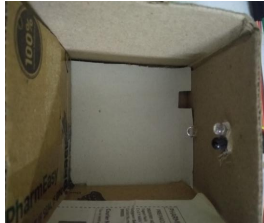
Fig.4: Close view how IR sensor is placed
