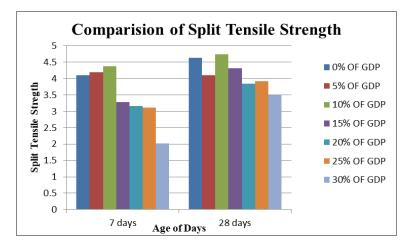
The above graph indicates that the split tensile strength for 7 and 28 days with 0%,5%, 10%, 15%, 20%, 25% and 30% replacement of GDP with cement. The strength increases for 28 days with 10% replacement of GDP when compared with normal concrete i.e., 0% replacement of GDP with cement.
