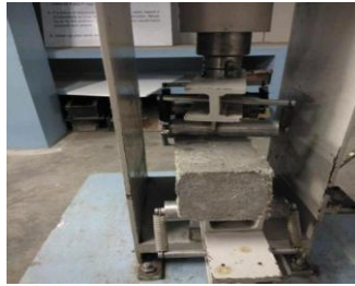
Figure 6 : Flexural Strength test setup
