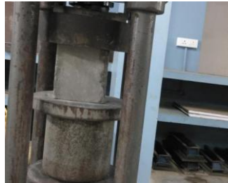
Figure 2 : Compression Strength Test Setup
