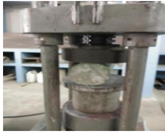
Figure 4: Tensile Strength test setup
