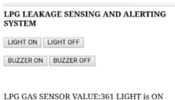
Fig 8: Gas Leakage Detection Displayed through Webpage.
