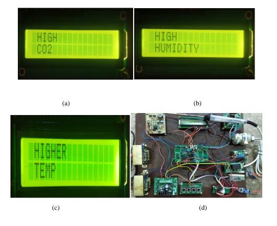
Fig. 5 (a) LCD display for high Co2 (b) LCD display for high humidity (c) LCD display for high temperature (d) Overall circuit
