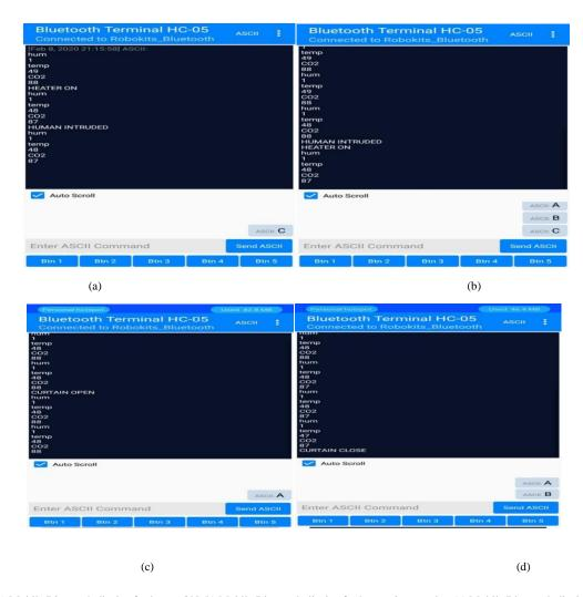
Fig. 3 (a) Mobile Bluetooth display for heater ON (b) Mobile Bluetooth display for human interruption (c) Mobile Bluetooth display for opened curtain (d) Mobile Bluetooth display for closed curtain
