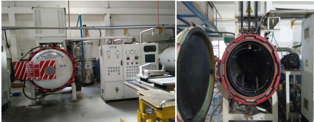
Figure 1 : Vacuum furnace used for sintering
