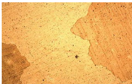
Fig. 3: Optical micrograph of FSW zones of PWHT joints T6 (190 0 C for 10h)
