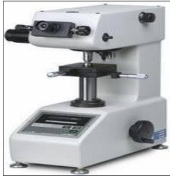
Figure 3: Vickers Hardness Tester
