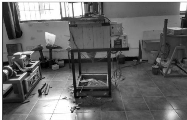
**Figure 1: Stir casting set-up assembly**
