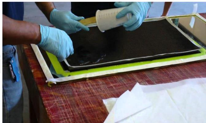
**Figure (a)** Sandwich Structure panel, **(b)** Preparation of face sheets
