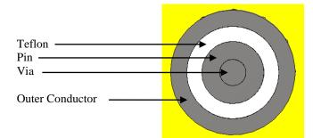
It consists of an inner conducting material, an insulating material and an outer conducting material. The inner conducting material has two parts via and pin, both are connected to the patch. They are made with PEC. The insulating material is made with Teflon (PTFE lossy in CST). The outer conducting material is also made with PEC and is connected to ground. The dimensions required for an SMA connector are:
