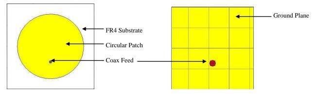
A patch antenna consists of patch, substrate ground plane and feed point. Ground plane and the substrate are taken in square shape with equal dimensions. The radius of the patch is calculated from the above equation. By adding 2 mm to it the sides of the substrate and ground plane can be obtained.
