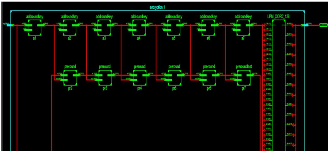
Figure 4: RTL view of proposed MAES algorithm
