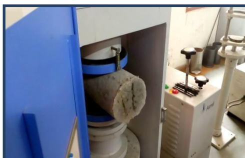
Figure 7: Split tensile Strength Testing
