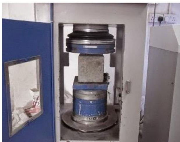
Figure 6: Compressive Strength Testing
