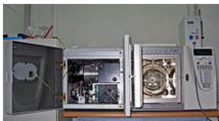
A GC-MS unit with doors open. The gas chromatograph is on the right and the mass spectrometer is on the left.
