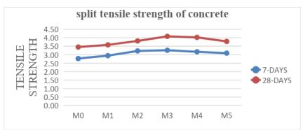
Split Tensile Strength of Cylindrical Specimens by Accelerated Curing
