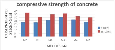
Compressive Strength of Cube Specimens by Accelerated Curing
