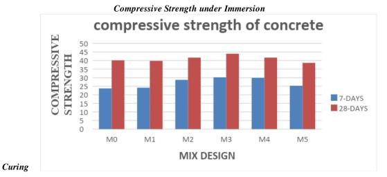
Compressive Strength of Cube Specimens under Gunny bag Curing
