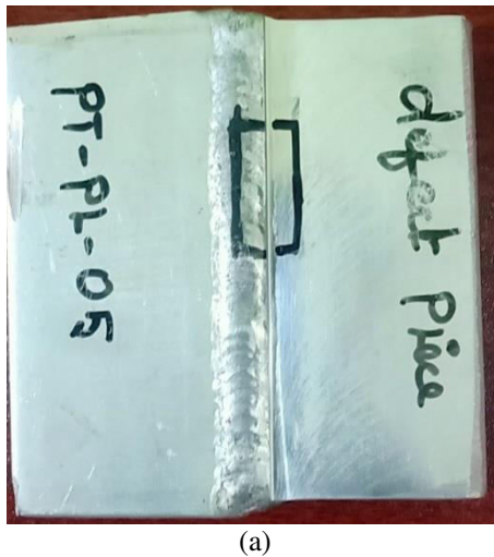
Fig7 (a) after cleaning the defect was found
