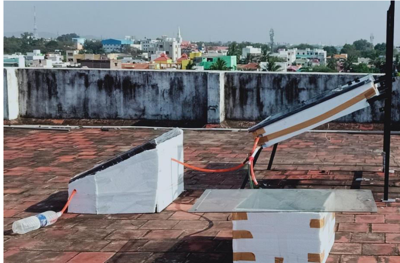
Fig 3 Inclined Still with basin still
