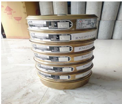
Figure 1 Sieve analysis test for fine aggregate
