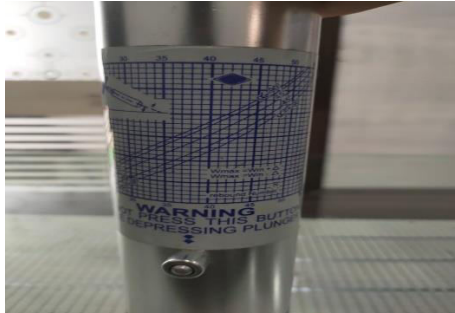
Fig.1 Rebound Hammer Graph
