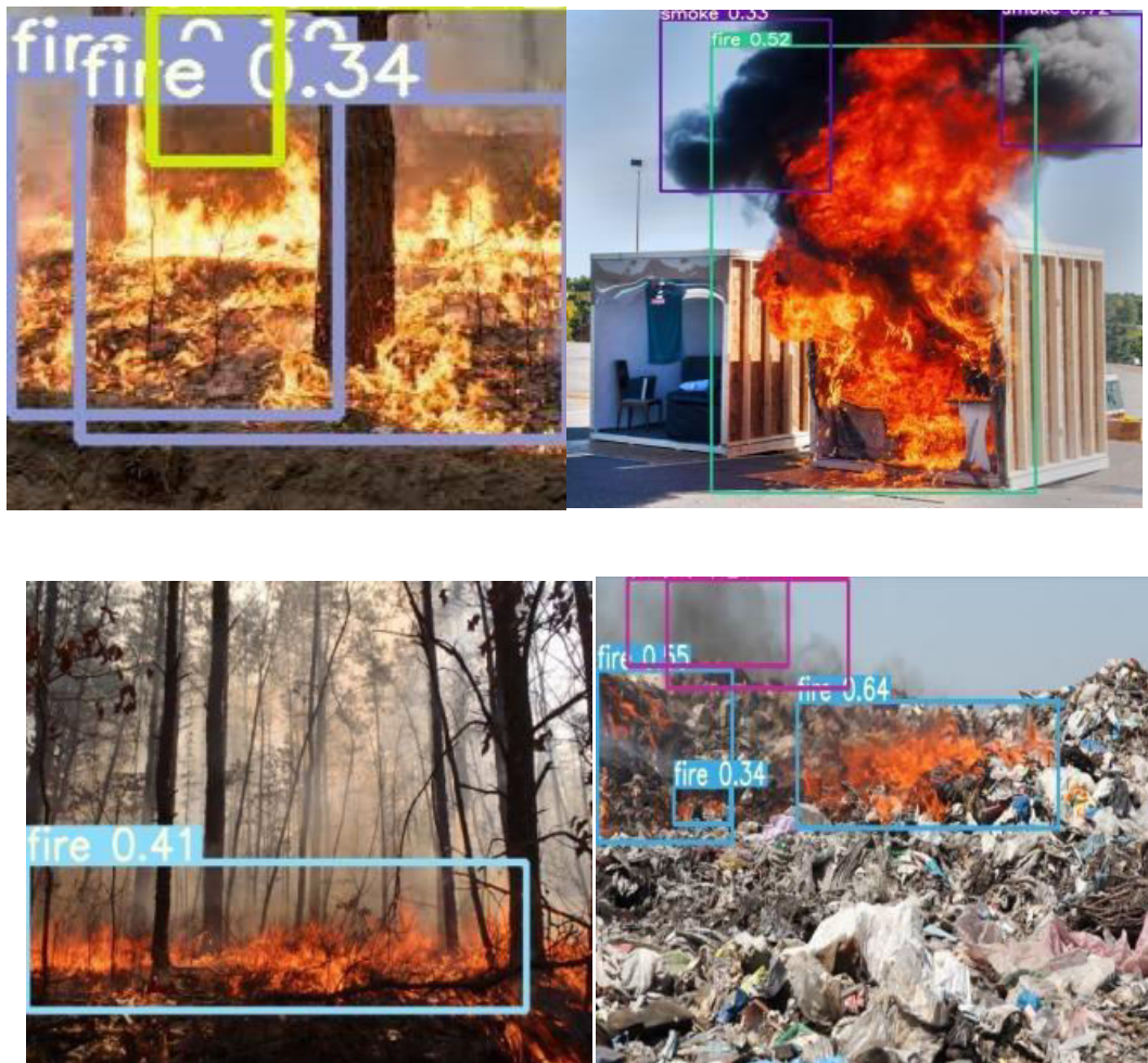
Fig 6: Fire Detected in images with Bounding box
