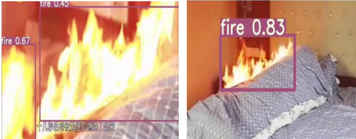
Fig 7: Fire detected in videos with bounding box
