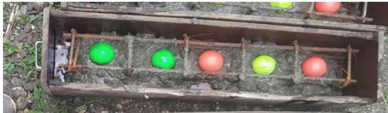
Beam Section with HDPE Ball
