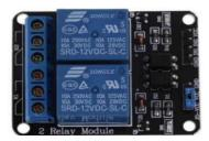
•12V 2channel relay board module can control various appliances and other equipment that draws large current. It can be controlled directly by microcontroller (raspberry pi, Arduino, 8051, avr, pic, dsp, arm, arm, msp430, ttl logic)
