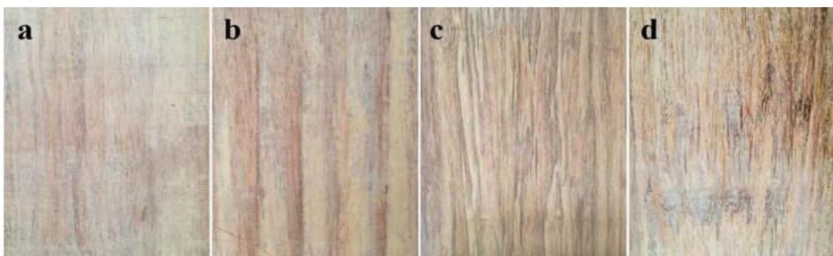
**Figure 6:**The surface of bamboo scrimber with different textures (a wood grain; b strip-shaped; c mountain-shaped; d pattern of vortexes) [7]
