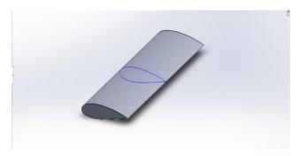
The design of Lockheed c-141 13% airfoil in SolidWorks by taking coordinates from airfoiltools.com. Steps:
