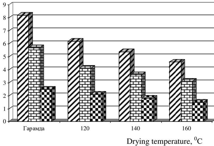
Figure 3. Changes in cleaning efficiency after the drying process of Ko'paysin selection cotton.
