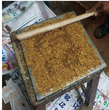
Fig. 4. Hand layup process of kora fiber impregnated in the polyester resin.
