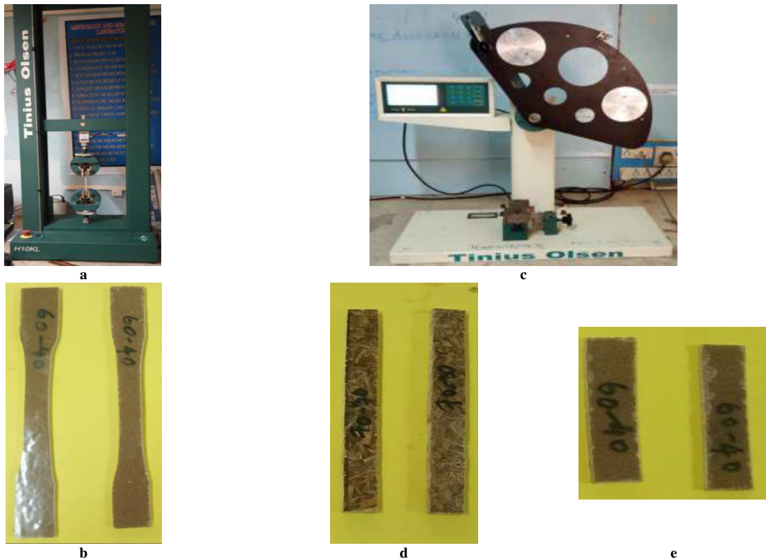
Fig. 6. Tensile tests (a) universal testing machine used to perform the tensile tests (b) impact tester (c) tensile specimens (d) flexural test specimens (e) impact test specimens.
