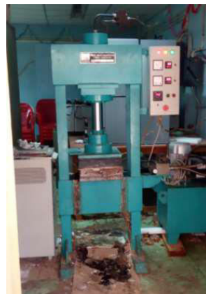
Fig. 5. Compression molding equipment used to fabricate the composite plate.
