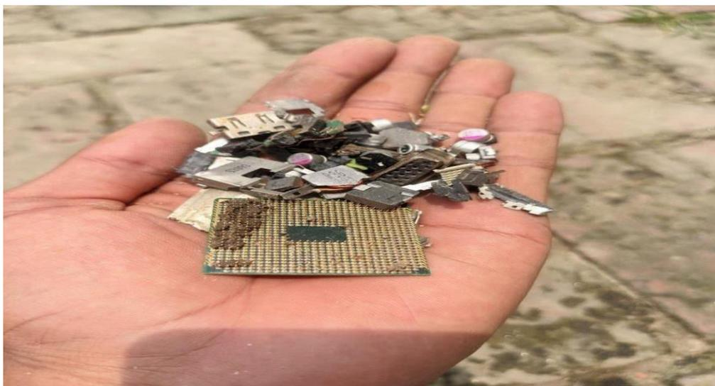
**Fig.1. electronic waste as coarse aggregate**
