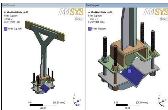
Figure 6:-Modified Design Of Blade CAD Model (fixed support)
