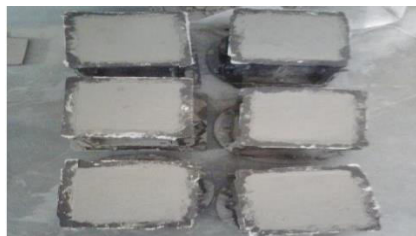
Ultrasonic Pulse Concrete cube casted in mould
