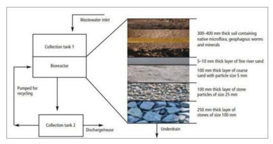
The overall duration for operation of treatment process is 4-6 hrs. The filter bed is then kept in rest for the rested time before the next cycle. In Soil Biotechnology system, problem of clogging is get overcome by propagating soil
