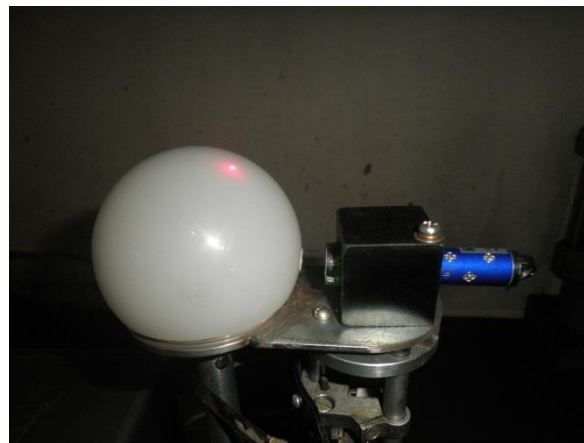
Fig. 5. General view of the laser head for measuring the vibration amplitude of the spindle tip.
