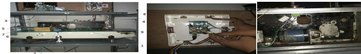
(a) Schematic of experimental setup and its component (b) Connection to ARDUINO Board (c) AC motor and Worm-worm Gear
