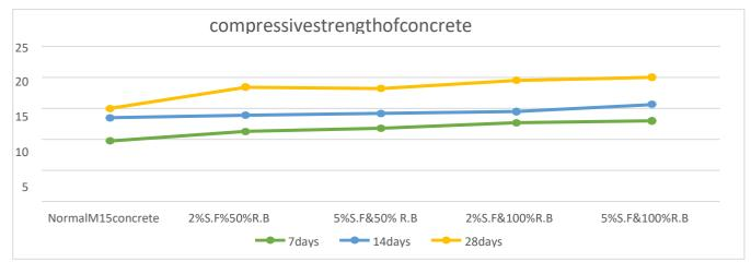
Figures shows the results of compressive strength text fornominal M15 concrete is 15 N/MM2,by using rations of fine aggregate and coarse aggregate partial replacement of robo sand and steel fibers. Figs. 2 shows the tensile strength test of concrete comparison of nominal M15 grade concrete and ratios of using the robo sand and steel fibers in the conventional concrete.
