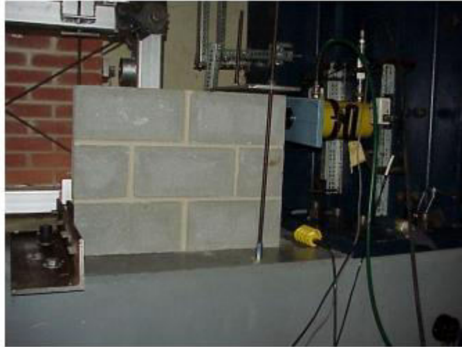
(Figure 4. In-plane, destructive shear test set-up.)
