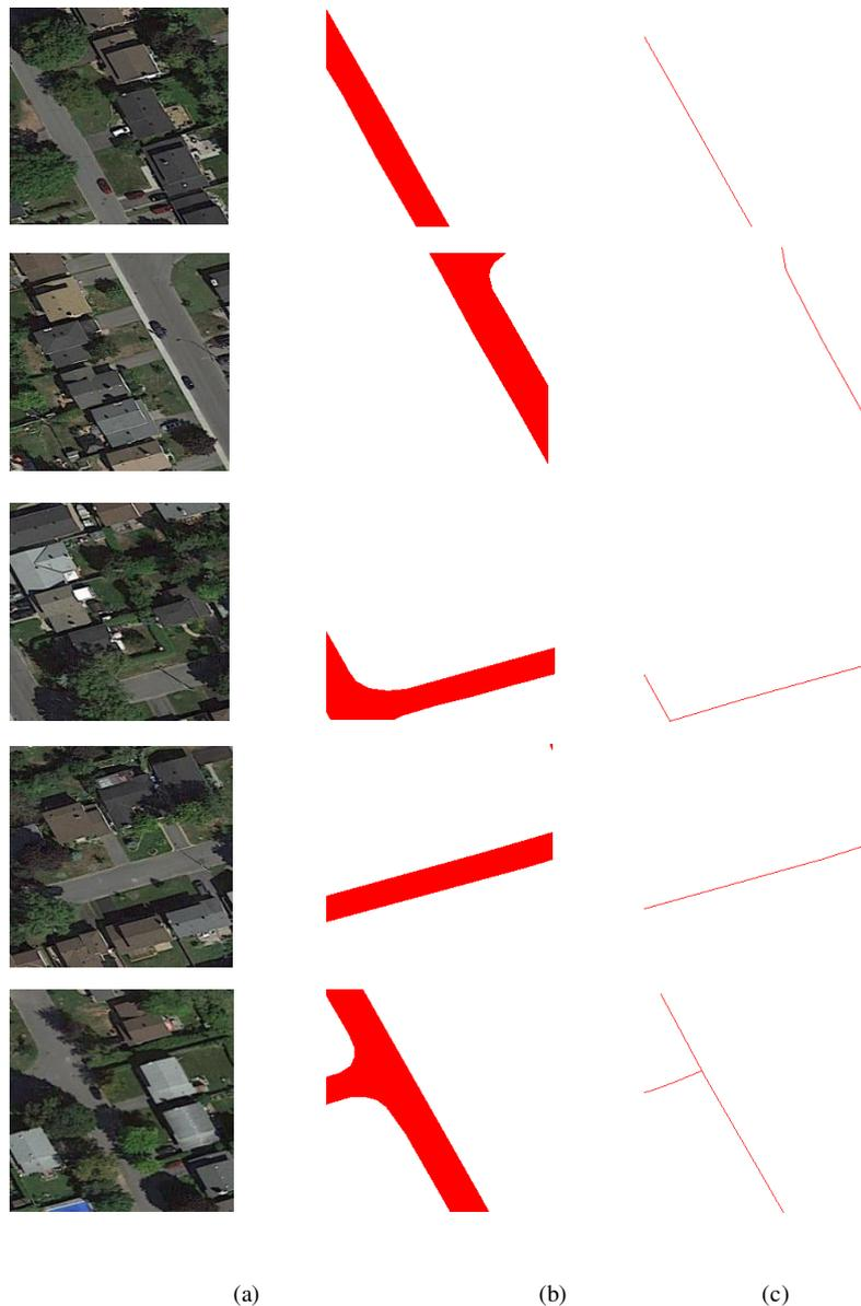
Fig. 4. Random input VHR images to be extracted from the dataset provided to the model. Images are complex and consist of challenges like shadows and occlusions by the trees and buildings. The content in the fig is (a) Input images for the testing purpose (b) ground truth of the road surface for respective input image (c) ground truths of the centerlines for respective road network images.
