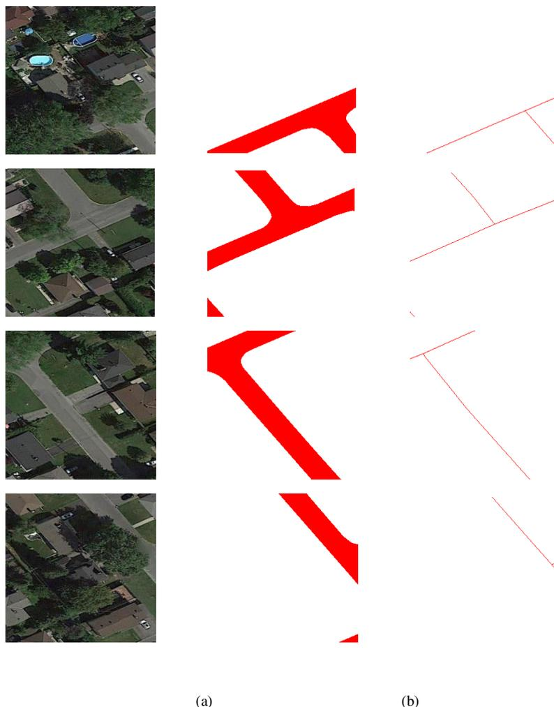
Fig. 3. Sample images from the dataset after cropping the dataset into  $256 \times 256$  dimensions for a) input images after cropping into  $256 \times 256$ . b) ground truth for road surface segmentation with dimension  $256 \times 256$ . c) ground truths for centerline with dimensions  $256 \times 256$ .
