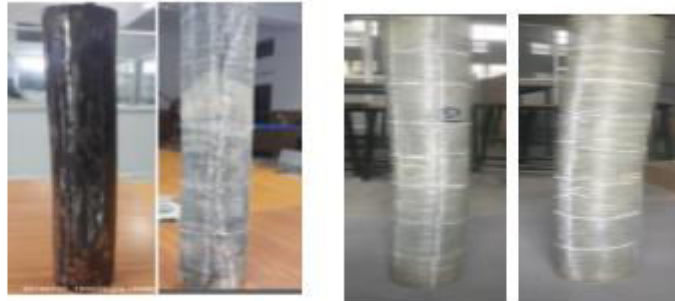
Figure 5 (a) Failure pattern for CC (b) Failure pattern for CG-1 (c) Failure pattern for CG-2 (d) Failure pattern for CG-3
