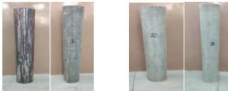
Figure 1 (a) Conventional Column CC (b) Strengthened Column with one layer CG-1 (c) Strengthened column with two-layer CG-2 (d) Strengthened column with three layers
