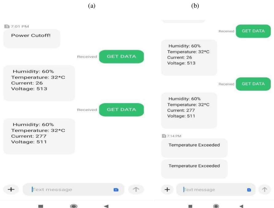
Fig. 1. Fault detection (a)SMS of Transformer health received after requesting the program via SMS. (b)Automatic SMS Alert Received by GSM
