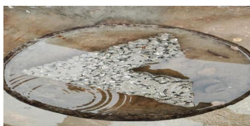
A-Shaped Interlocking Tiles curing
