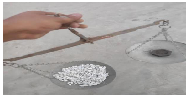
4kg Epoxy Coated Aggregate
