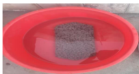
Hexagonal Interlocking Tiles curing
