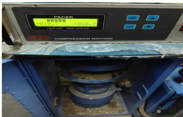
Compressive strength Test
