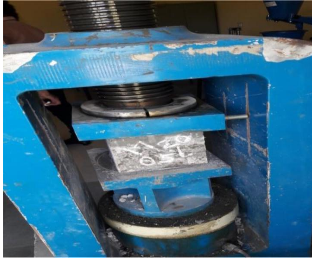
(Fig.3.6 : Experimental Setup of concrete Cube M20 (0.5% Polypropylene Micro Fibre))
