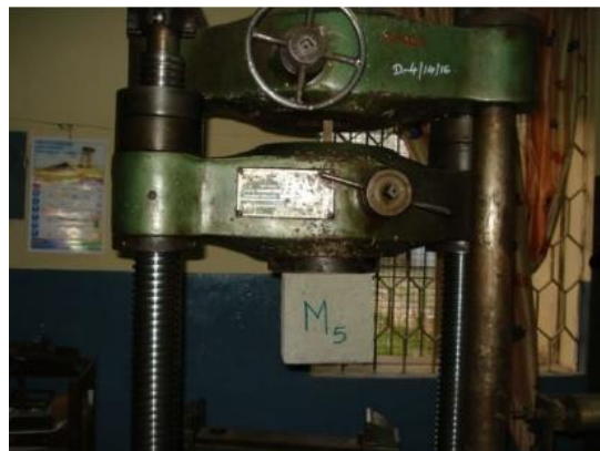
(Fig.3.5: Experimental Setup of concrete Cube M20 (1% of Fibre))
