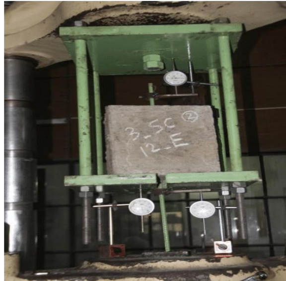
(Fig.3.4: Experimental Setup of concrete Cube M20 (1% Polypropylene in Concrete))
