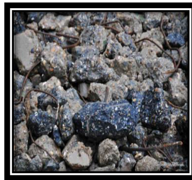
fig.b. Waste Aggregate of demolished building
