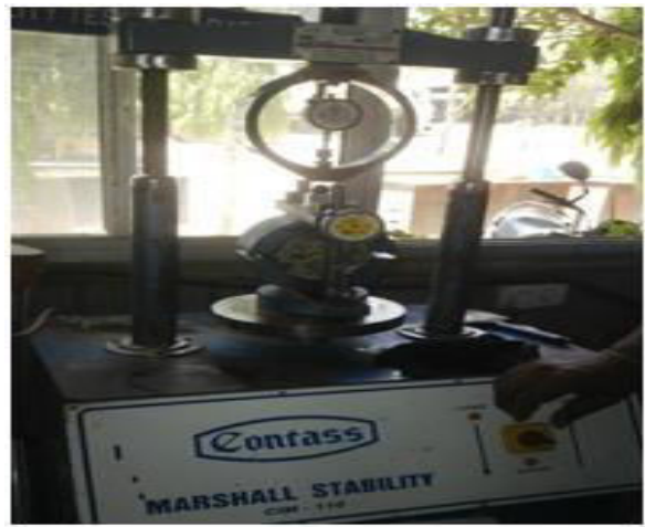
fig.5.2 Marshal Stability Testing
