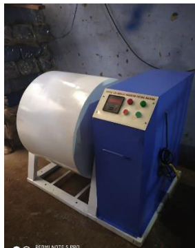
Fig.6.1 Los Angeles Abrasion Test Apparatus
