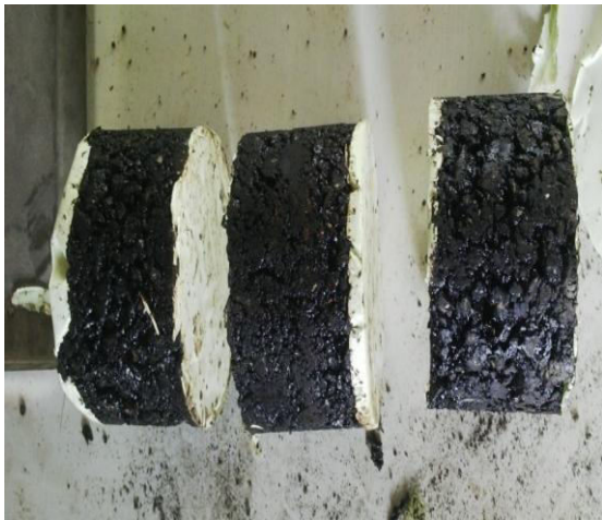
Fig.5.1 Marshal Stability Test Specimen
