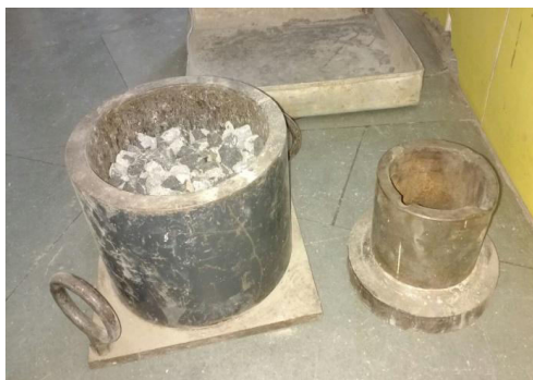
Fig.2.1 Aggregate crushing value test apparatus
