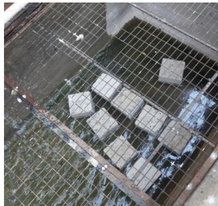
Figure 2. Curing of blocks
