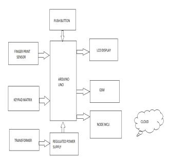
The system uses a fingerprint sensor, Node MCU, arduino, GSM, regulated power supply, Transformer, push button and LCD.
